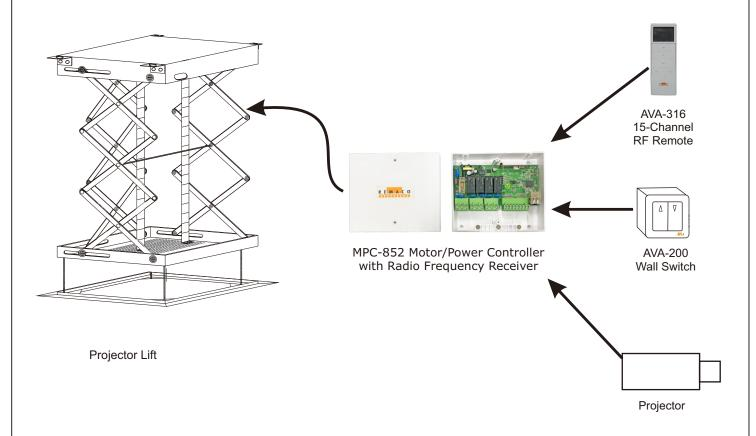
△ Connection of all cables to the MPC-852 (Refer to Installation Guide of MPC-852)
