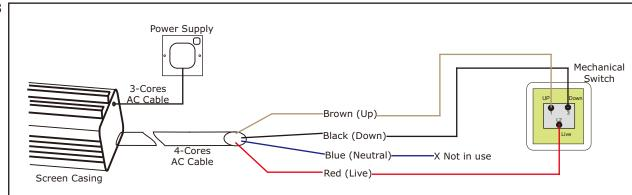
E) Terminate AC cable as shown in figure.
